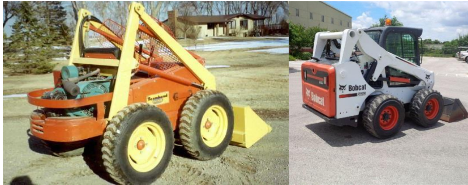
M400 (left) and S650 (right) showing the evolution of the bobcat Skid Steer Loader
