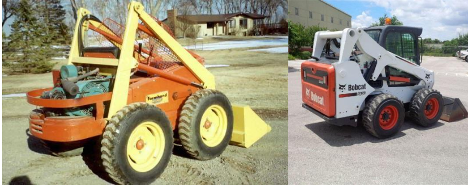
M400 (left) and S650 (right) showing the evolution of the bobcat Skid Steer Loader
